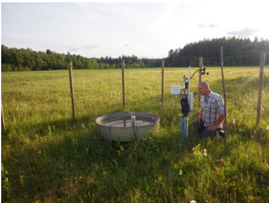
Photo 130: Measurement station with evapotranspiration measuring container (photo by E. Gutowska).
