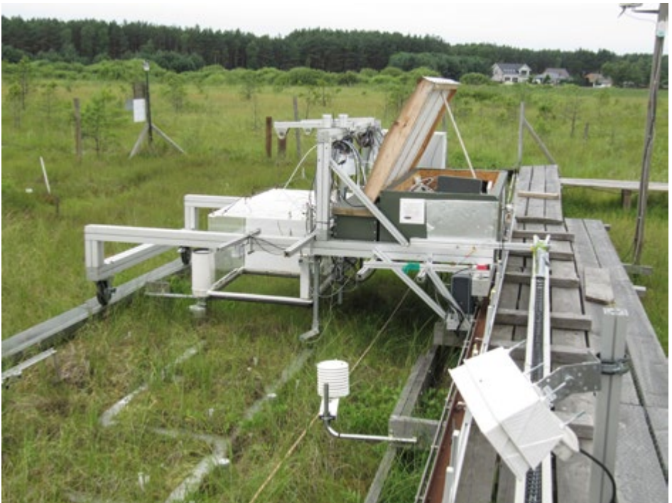
Photo 87: An automatic measuring station for the balance of greenhouse gasses, a manipulation experiment in Rzecin mire (photo by J. Kujawa-Pawlaczyk).
