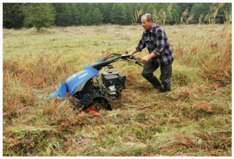
Photo 62: Single-axle tractor – rubber track cylinder mower, perfectly coping with the most difficult conditions on a strongly hydrated fen, is a very good and effective technical solution. At the same time, it allows to mow an area about 4 – 5 times larger than that of a petrol brushcutter, using about 2/3 less fuel and causing little damage to the vegetation (photo R. Stańko).
